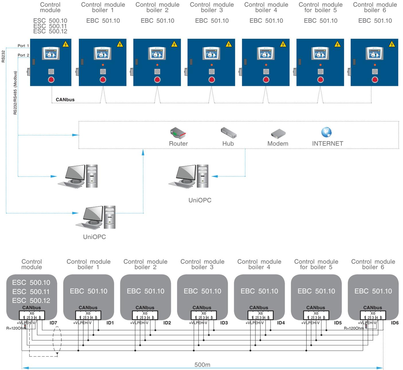
SP201. CANbus connection diagram ESC 500.10, ESC 500.11, ESC 500.12
