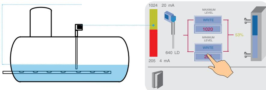
When filling the deaerator with water, bring the deaerator level to the minimum value (according to the deaerator datasheet) and write down the digital value of the minimum level.
