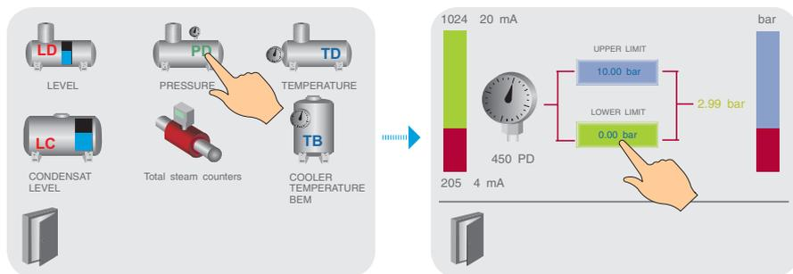
To set up the pressure sensor, enter the values of the sensor's lower and upper limits according to the datasheet.
