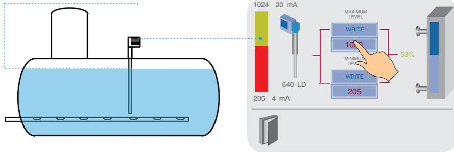
When filling the deaerator with water, bring the deaerator level to the maximum value (according to the deaerator datasheet) and write down the digital value of the maximum level.
