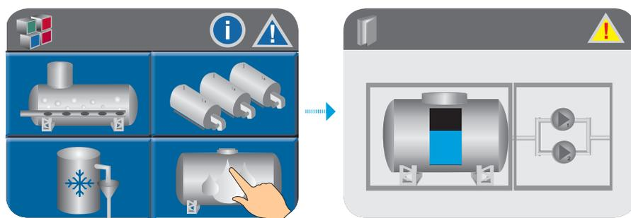
To go to the feed water deaeration control system from the main menu screen, press the condensate tank icon.
