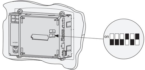
The jumper settings shown above determine the controller's ability to perform the functions of the terminal device in the RS485 network. Please note that the default factory setting is YES. If the OPLC (operator's PLC) is not a terminal network device, install both jumpers in the NO position.
