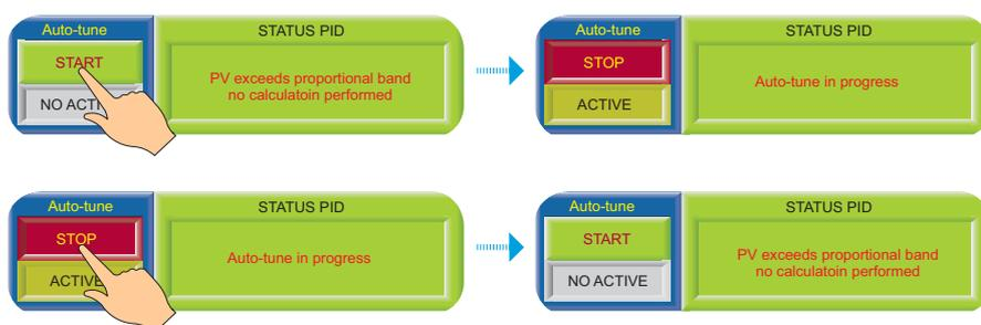
Auto-tune can only be performed with the burner being in operation. Press the START button on the screen to begin the auto-tune process. Press the STOP button to stop the auto-tune process.
