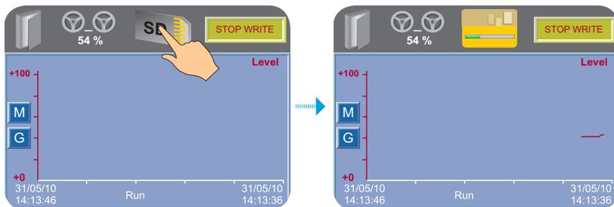
Insert the memory card into the slot. Run the trend by pressing the START button and then press the memory card icon — the trend will begin to write to the SD card. If the trend is deactivated, writing to the SD card will be stopped automatically.
