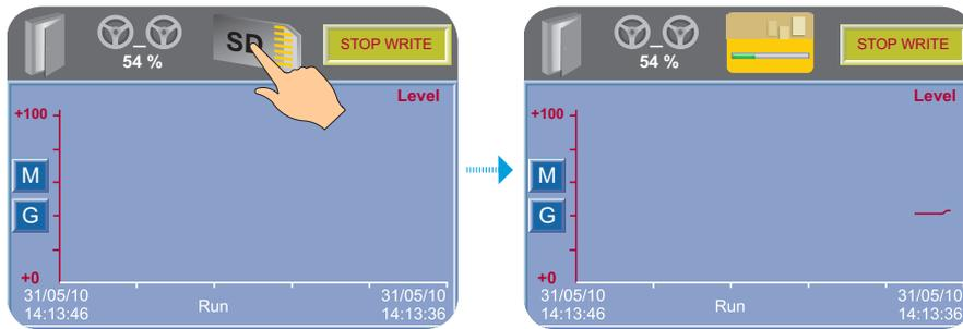
Insert the memory card into the slot. Run the trend by pressing the START button and then press the memory card icon — the trend will begin to write to the SD card. If the trend is deactivated, writing to the SD card will be stopped automatically.
