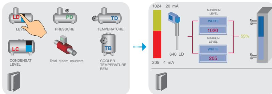
The level sensor setup is performed after being installed on the deaerator.
