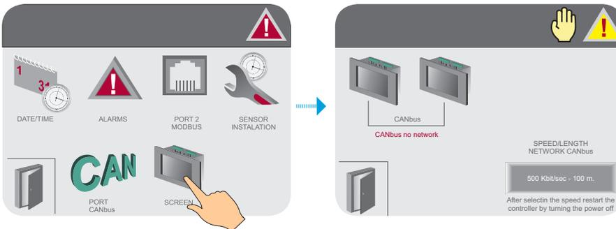
The CANbus network is designed for cascade control of steam boilers. The network setup consists of selecting the data transfer rate, which shall be the same for all systems connected to this network. The transfer rate itself depends on the extent of the network, which is determined by the route length of the network cable laid from the two outermost control systems as shown in the figure below.
