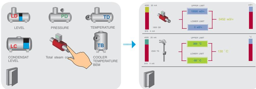
To set up the temperature sensor and the flow-meter, enter the values of the sensor's lower and upper limits according to the datasheet.
