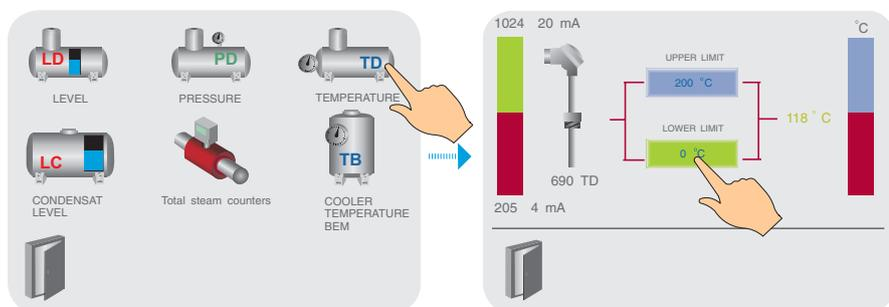
To set up the temperature sensor, enter the values of the sensor's lower and upper limits according to the datasheet.
