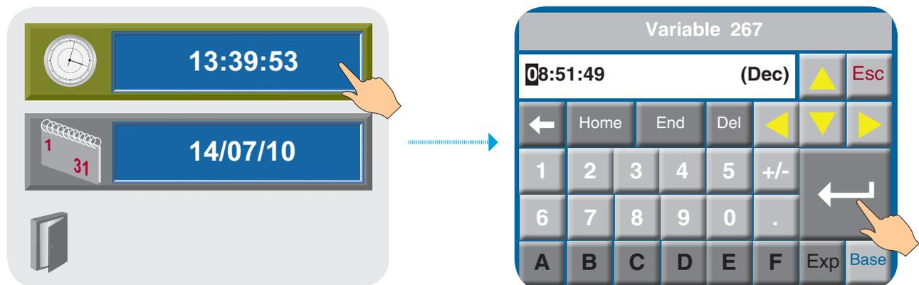
Press the time or date entry box → Enter the necessary value on the keypad and press Enter.
