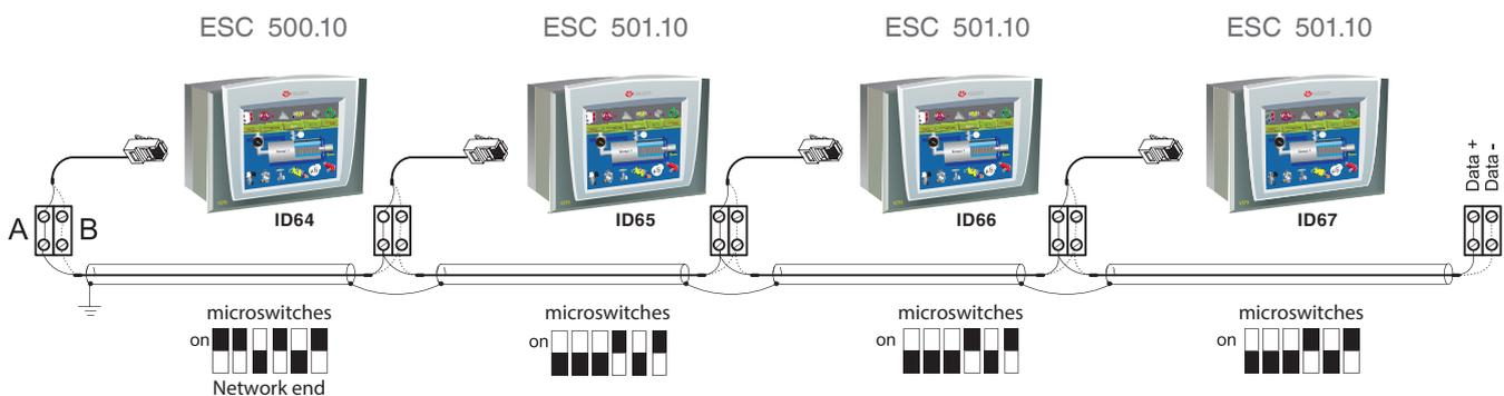
Do not establish conditions where positive (A) and negative (B) signals intersect. Positive outputs shall be connected using positive cables and negative outputs using negative cables.
