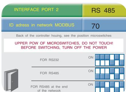
Port 2 is used to connect the ESC to the Modbus network.
