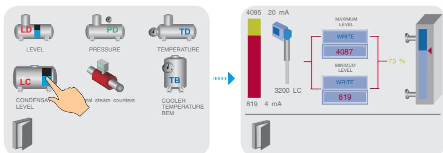
The level sensor setup is performed after being installed on the tank. Before filling the tank with water, the digital level indication on the screen shall display a value of no less than 205+3, which corresponds to the sensor 4 mA current signal.\*
