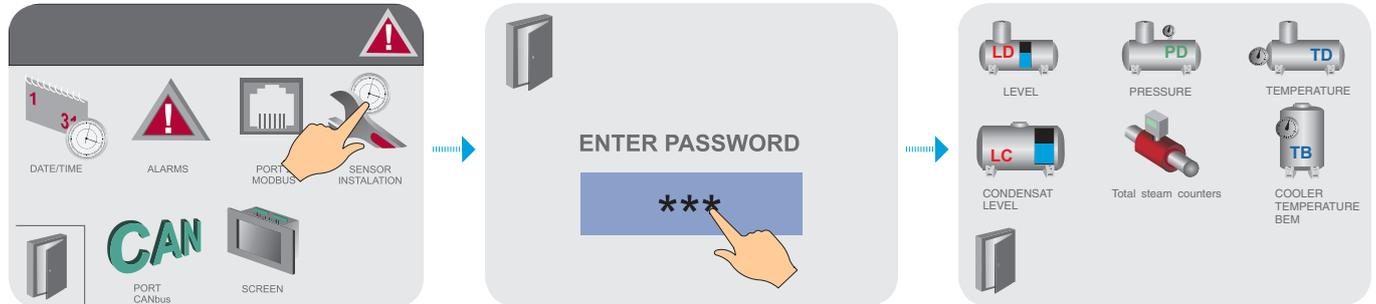
**i** Depending on the ESC configuration, unnecessary sensors will be hidden.
