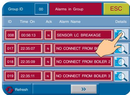
The alarm is unacknowledged ▶ Press to acknowledge
